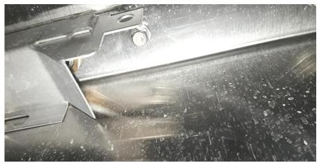
This picture is showing a normal setting. Properly adjusted, the diverter duct would only send a small stream of water into the rinse tank, approx the size of a pencil. This adjustment would fill the rinse tank after the wash tank overflowed into and filled the scrap tank.
