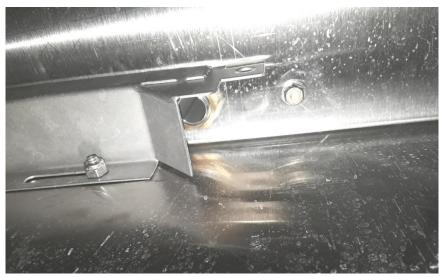
By moving the deflector so it covers half the pipe exit tube, water would be deflected towards the rinse tank.
