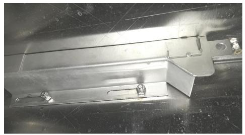
Please note in picture #1 looking up, the adjustment studs are shown at the far right of the slots (meaning the diverter duct is moved to the far left for this machine--a R-L conveyor) and the water pipe exit is fully open to drop into the wash tank. Adjusted as shown means the rinse tank would receive no water and the machine would continually fill, not shutting off.
