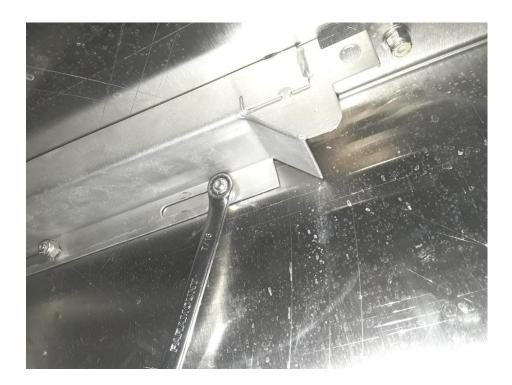
How to adjust the diverter duct, loosen both nuts holding the plate to slide left or right
